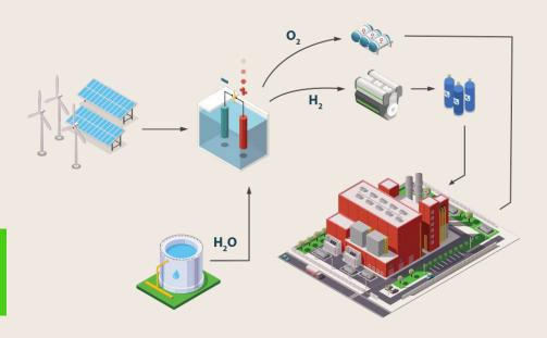
Generate hydrogen where you need it with an on-site electrolyzer powered by renewable energy.
